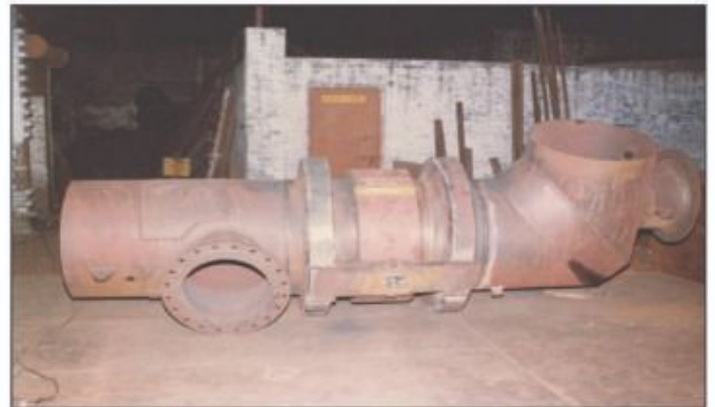
Cross Around Pipe Assembly
