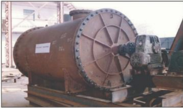
Dry Melter with Stirrer for cooking
