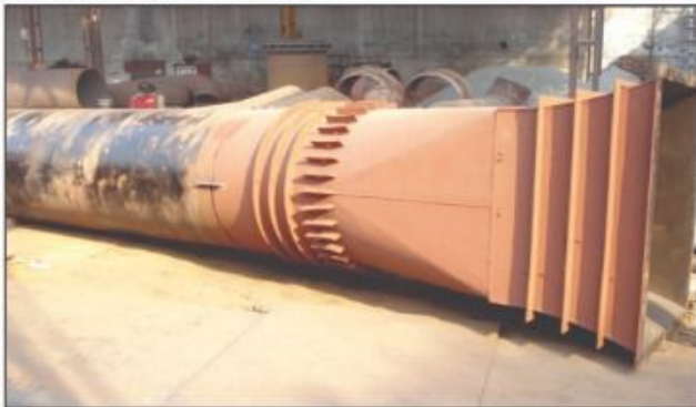
Bell Mouth with connecting Penstock Pipe
