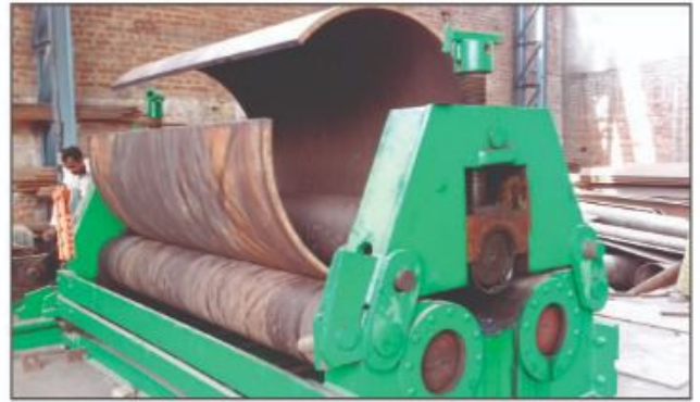
Rolling of High Yield Strength Plate
