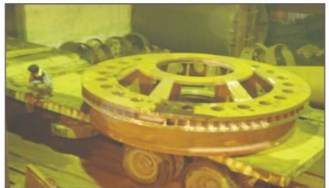
Turbine Top Cover for Hydro
