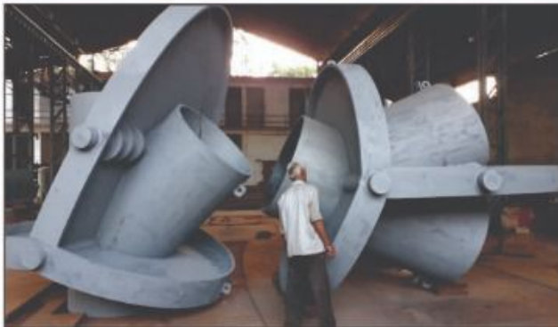
Bifurcation Pipe with Tie Rods
