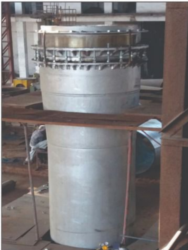
Expansion Joint of Length 5000 mm
