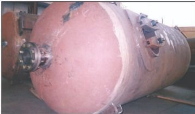
Air Receiver - Test Pressure 63 Kg / cm 2
