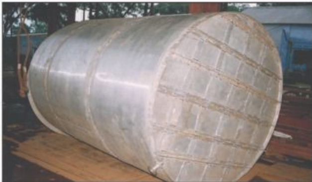
Aluminum Tank for H 2 O 2 storage for Paper Industry
